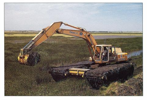
The department's amphibious backhoe is used to dig the level ditches, which will hold deep water for strorage and create additional wildlife habitat.
